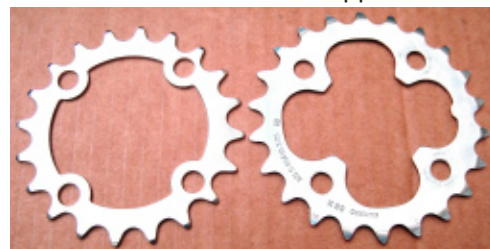
Comparison of 20T (left) chainring with 22T
